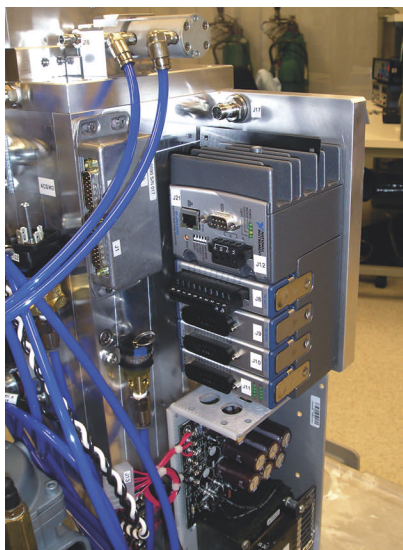
The Visica 2 cryoablation system for the treatment of tumors (left, courtesy of Sanarus) went from a requirements document to first revenue in 14 months, according to systems engineer Jeff Stevens. Stevens used LabView to develop code for the CompactRIO platform (right, courtesy of National Instruments) that served as the embedded engine in the Visica 2.
