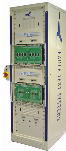
The ETS-88 supports multi-application operation and combines four independent mixed-signal testers in a box. Each mini tester can drive its own handler or prober.
