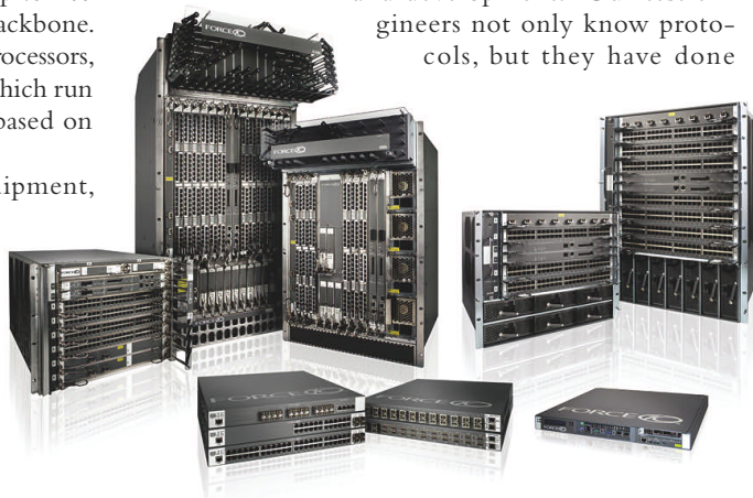
FIGURE 1. All switches and routers from Force10 Networks, regardless of configuration, share a common code base.
